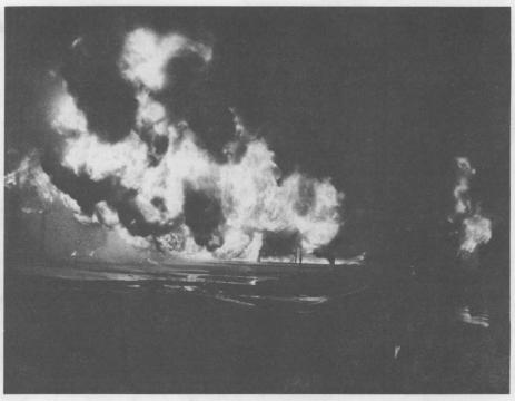
building up at the ceiling. In photo at right, some two to three minutes after ignition, the building — by now a raging inferno — burns end to end.
